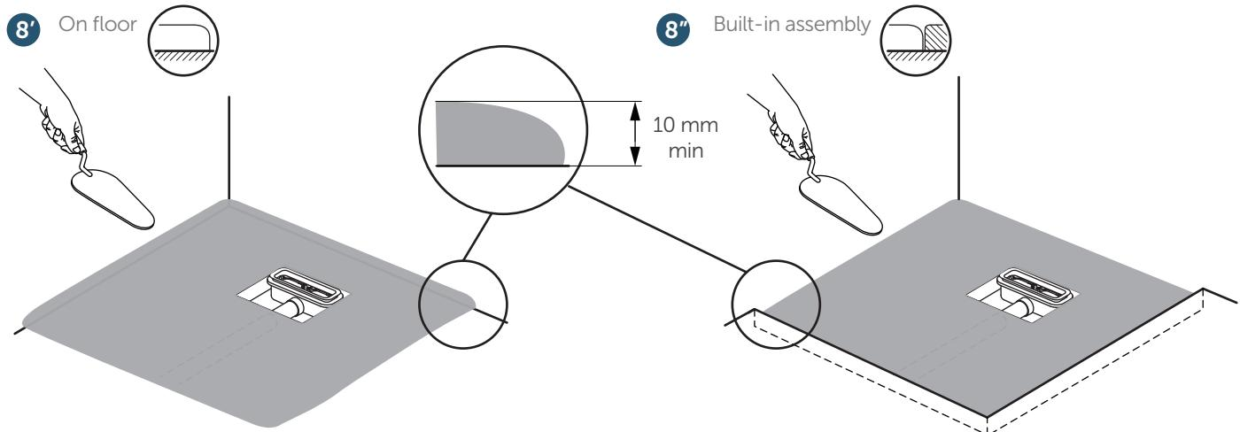
Mix the Solvent Free, Cement Based Flexible Tile Adhesive in accordance to the manufacturers instructions to a workable mix to cover the total area under the tray. Trowel to a thickness suitable to allow levelling and support of the shower tray.
